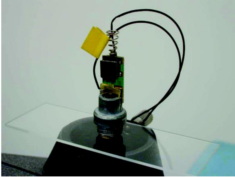
Fig. 8. Disassembled laser pointer mounted to the microscope camera port
