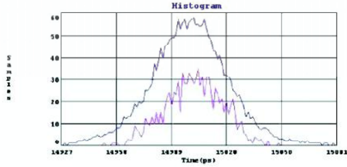
Fig. 2. APEX intrinsic jitter performance for 1,000 clock samples (bottom curve, peak-to-peak value 97.0 ps, \sigma_{\text{jit}} \approx 15.9 ps) and 1,000,400 clock samples (upper curve, peak-to-peak value 151.4 ps, \sigma_{\text{jit}} \approx 15.7 ps)
